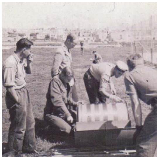
Lt Anderson RE unwinding the measuring tape from the drum; Marsa Sports Ground.
