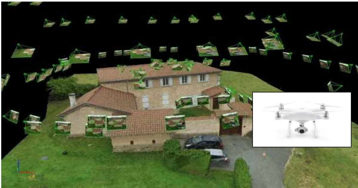
A snapshot of a 3D model, created from multiple stills taken by a small COTS UAV currently being trialled by 42 Engr Regt (Geo) (image courtesy of Pix4d)
